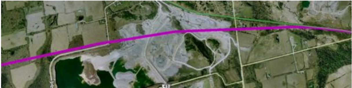
**Figure 5 Climbing the escarpment - the ground rises 40 metres from right to left. The railway will run across a gravel pit on a new embankment, then into a cutting on the high ground.**
